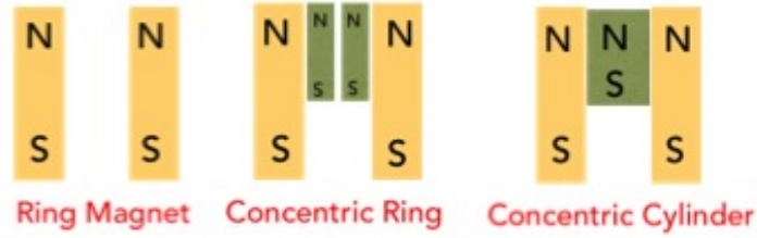
Figure 3.8: Cross-sectional view of different magnet assemblies tested. Here N and S represent the magnet poles. IR - Inner radius, OR - Outer radius, H - Height
